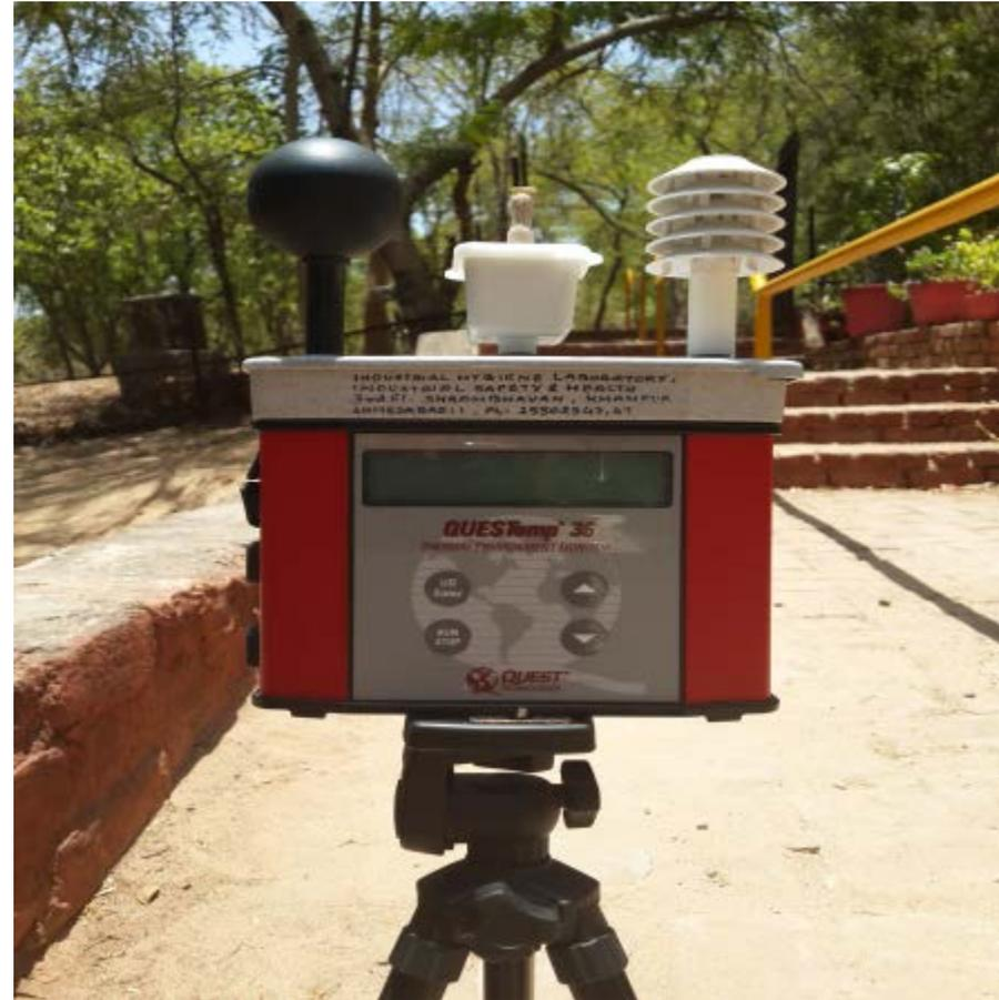
WBGT instrument used for temperature measurements across the city
